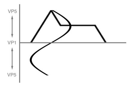
Envelopes are unipolar modulation signals. The modulation starts at the vowel adjusted with the Vocal Position control and proceeds to step through the vowels depending on the adjusted intensity.
