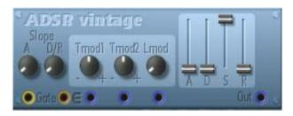
completes, and the modulation falls back to the sustain level. The time needed for this is the decay time. A decay will not be heard if the sustain level is set to maximum.
