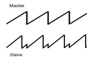
Normally you would connect the Sync Out of a SyncMaster to the Sync In of the slave(s). Then use a pitch modifier (see under Modifiers) to modulate the pitch of the slave(s) using any modulation signal.
