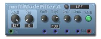
frequency relationship to the pitch across the entire keyboard. At a setting of 50%, the cutoff frequency ratio will be lowered by 50% per octave above E3, and raised 50% per octave below E3. A value of 0% means there is no keyfollow modulation, and the cutoff frequency remains fixed.
